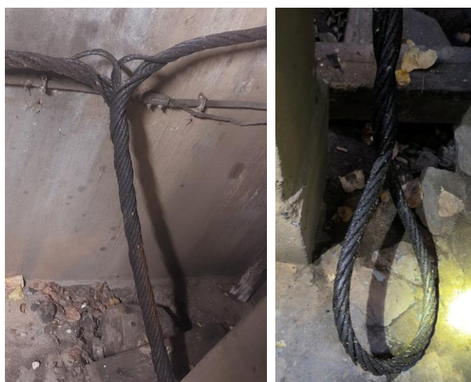
Fig. 13 - Loop formed by the post-fracture coiling of the cable.
